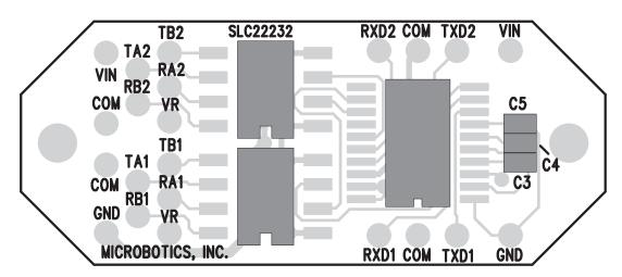
Each of the pads above (small, grey circles) represents an electrical connection on the board. The label next to the pad indicate the signal it connects. The left side of the board is for RS-422 connections. The right side is for RS-232/TTL connections.
