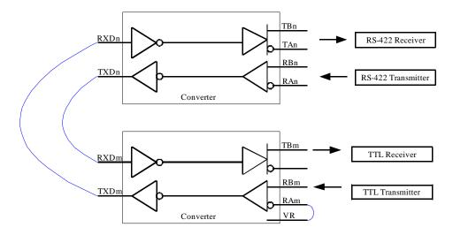
In the case of TTL connections, the serial converter must share a common ground with the TTL device. Also, the on-board reference must be tied to the inverted line of the RS-422 receiver. This allows the receiver to operate correctly with a single TTL input.
