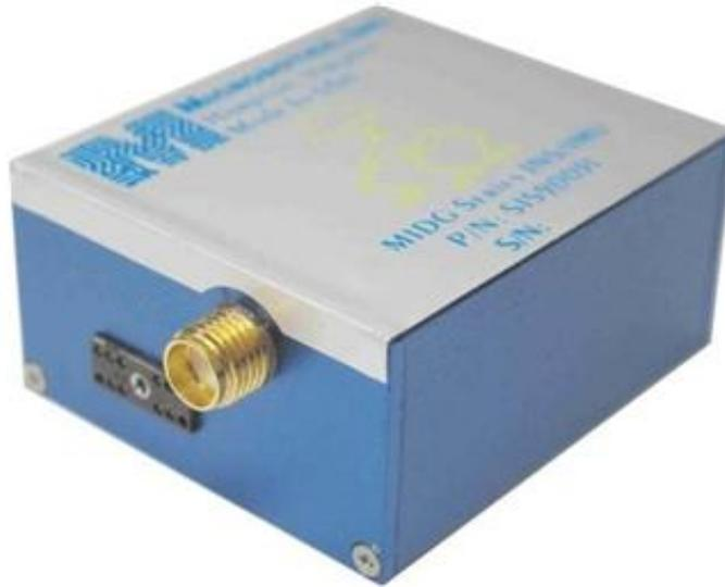
The MIDG IIC is a GPS aided inertial navigation system (INS) for use in applications requiring attitude, position, velocity, acceleration, and angular rates for navigation or control. An internal GPS receiver measures position and velocity and passes this information to the data fusion processor to be combined with the inertial data to generate an optimal solution. An internal three-axis magnetometer provides a magnetic heading reference when needed.
