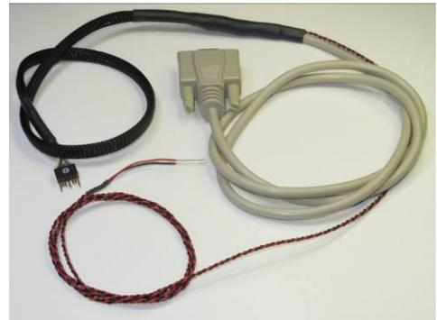
Figure 15. SLC2J09SF MIDG Series INS/GPS Interface Cable.
