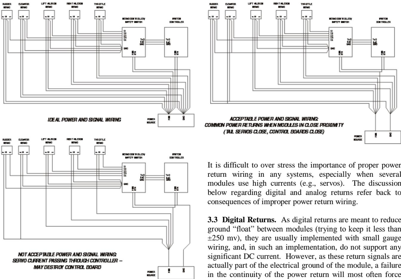
It is difficult to over stress the importance of proper power return wiring in any systems, especially when several modules use high currents (e.g., servos). The discussion below regarding digital and analog returns refer back to consequences of improper power return wiring.
